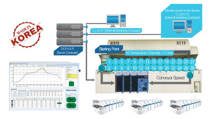
The System uses max. 32 channels temperature sensor fixed within the reflow to detect any temperature changes and evaluate its status real-time, while proximity sensors and photo sensors measure and monitor production environment of the reflow by detecting velocity of the conveyor and PCB. This enhancing productivity and preventing mass defects. The equipment can be maintained real-time from remote location via network version.
